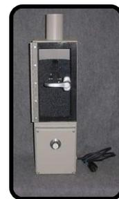
The **Zip Gravity** 3" and 4" stations are 7 1/2" W x 7 1/2" D x 26" L and weigh 38 lbs while the 6" station is 10" W x 10" D x 26" L and weighs 42 lbs. Each station requires no action from the user except to drop the carrier down through the iris of the station. At that point, the carrier uses natural gravity to drop down to the station below. No blowers or pushbuttons are used with the **Zip Gravity** station.
