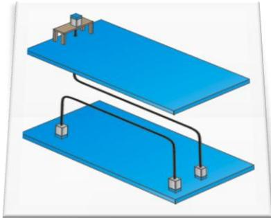
The “**DO IT YOURSELF**” pneumatic tube system is simple and economical to install and operate. Using our **Zip Basic** stations on each end of the system, connected by Schedule 40 PVC piping, couplings, and bends; you have a complete working tube system at your service.
